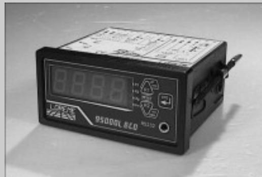
95000L BCD is a numeric indicator allowing to display a BCD value composed of 1 to 3 digits 1/2 unsigned or 1 to 3 digits signed. The personalization of the indicator, number of digits, sign, and input process configuration, active (voltage level) or passive (dry contact), allow to meet appliance majority. More, a configurable analogical output adds to indicator an analogical/numerical converter function.
